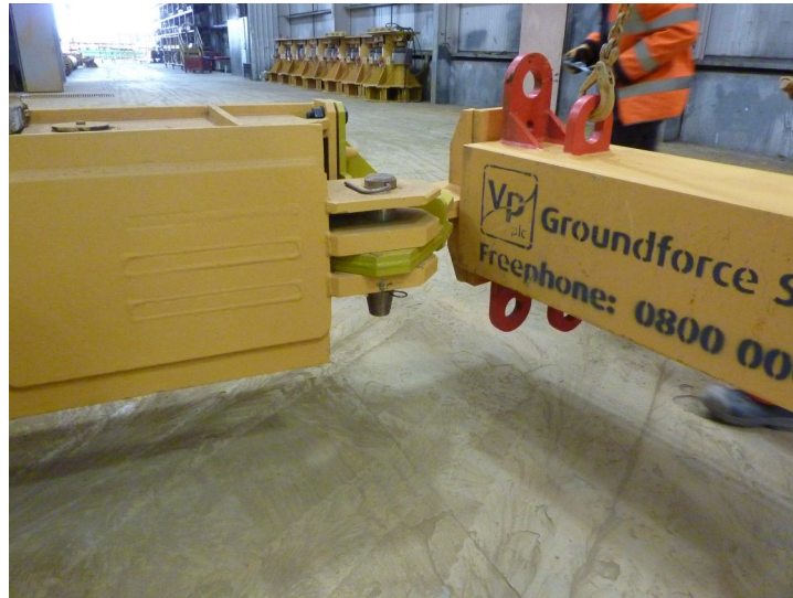
Image showing a Mega Brace hydraulic ram unit connected to a Super Mega Rough Adjuster.
