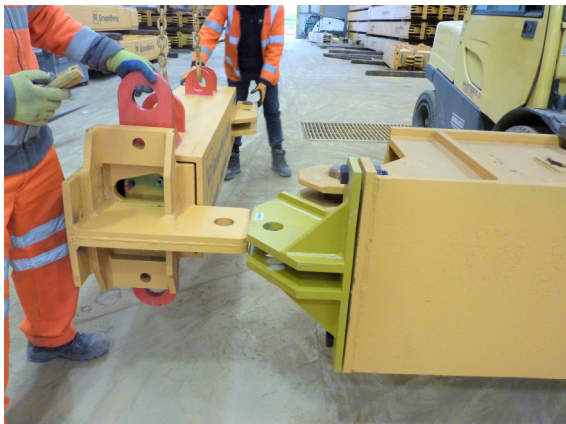
4. Once assembled, the Mega Brace hydraulic ram unit can then be connected to the Rough Adjuster End Adaptor.
